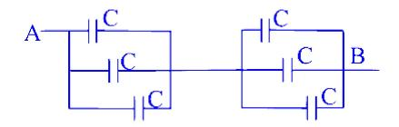
Thus, the parallel capacitors are calculated as  $C_p = C + C + C = 3C$
